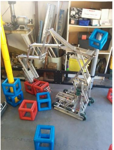
Because of this we instead built a reverse double four bar, powered by 6 motors and driven with a 7:1 reduction. This was a huge improvement in speed, reliability and maximum height compared to the previous scissor lift. The lift is easily able to reach over a full skyrise, and lifts to full height very quickly. Another advantage of the reverse double four bar is that it is linear, the intake does not move back or forward as the arm travels through its range of motion.
