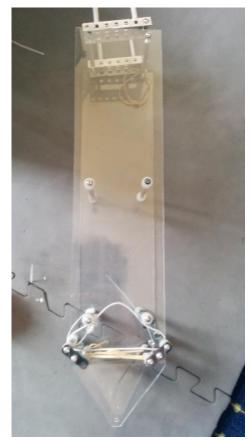
To build this we used 3D printed parts. Both of the allowed large 3D printed parts are used to make the tip of the needle, one of them being a nose cone and the other being the mechanism for the teeth that hold the cubes onto the needle.
