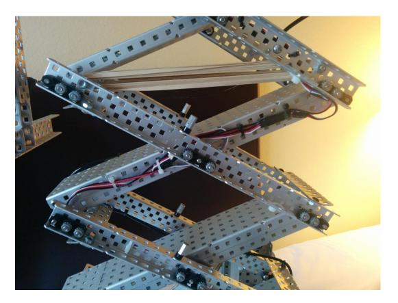
The winch scissor works by having a large driven gear on a tower at the back of the robot. This gear is attached to a spool that uses strings to pull the lift up and down as the winch is wound. The string to raise the lift runs straight off the spool and is connected to the bottom arm, and string to lower the lift is run from the spool, and around a roller at the bottom front of the robot.
