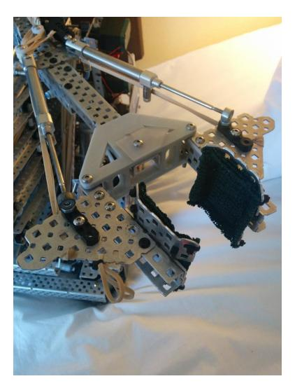
Because Mcchicken was a 15" robot, the swing arm had to fold back to be within size limit. To accomplish this, we used a hinge and latch arrangement, which is rubber banded to unfold when the robot lifts at the beginning of the match.
