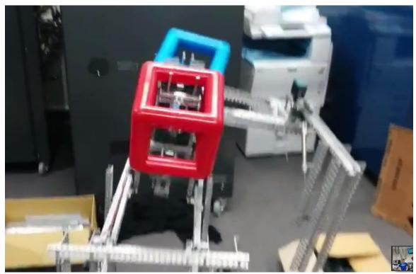
A solution to this was a skyrise manipulator on a chain bar arm, which would be mounted on the robot's centreline towards the back of the intake and swing over the robot from front to back. The pictured mechanism was built, but it was much too heavy so instead of putting it on the robot we decided to leave the problem until we could build a skyrise manipulator from lighter materials (3d printed plastic and/or plastic block).
